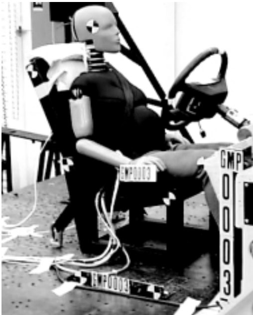
FIGURE 6 MAMA-2B set up for sled test impact simulation of frontal crash.
