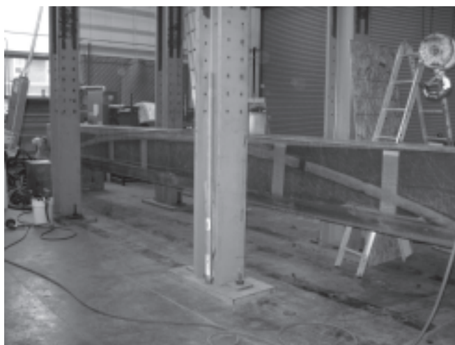
Hillman composite bridge beam is prepared for testing under a project funded by NCHRP IDEA and High-Speed Rail IDEA.
