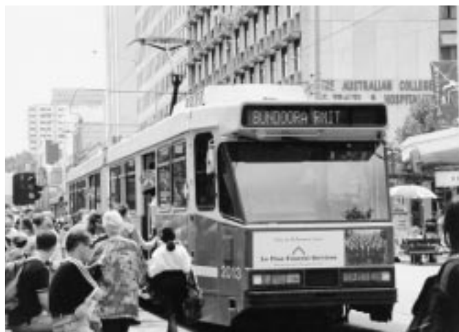
Melbourne Class B articulated cars, of which 132 are in service today. First ordered in 1983, they are equipped with chopper control and regenerative brakes. (Photo courtesy of John Gerofi.)
