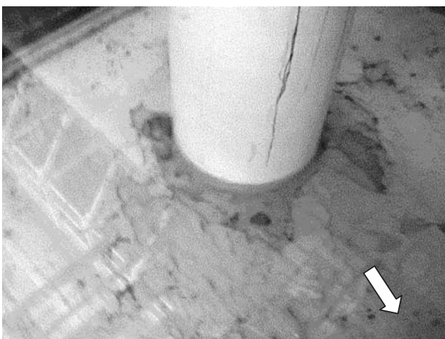
Figure A3 Pier Scour Hole under Shallow Water Condition—Back View.
