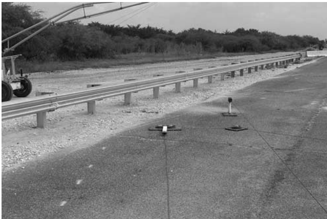
Figure 31. Modified G4(1S) before tests 472480-6 and 472480-7.
