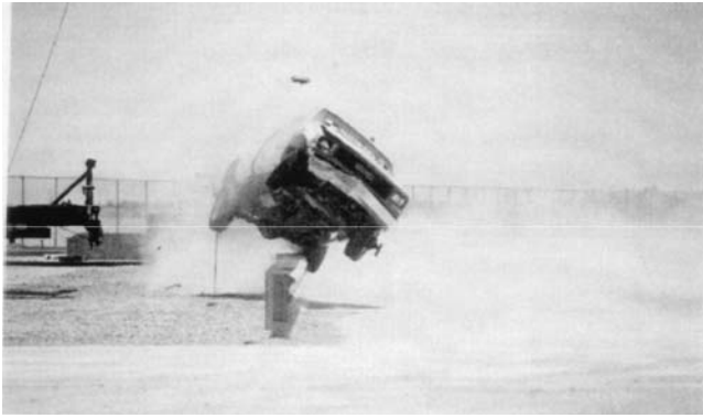
Figure 14. NCHRP Report 350 Test 3-11 impact with modified G4(1S) guardrail with nested 12-gauge W-beams and a 102-mm curb under the rail (32).
