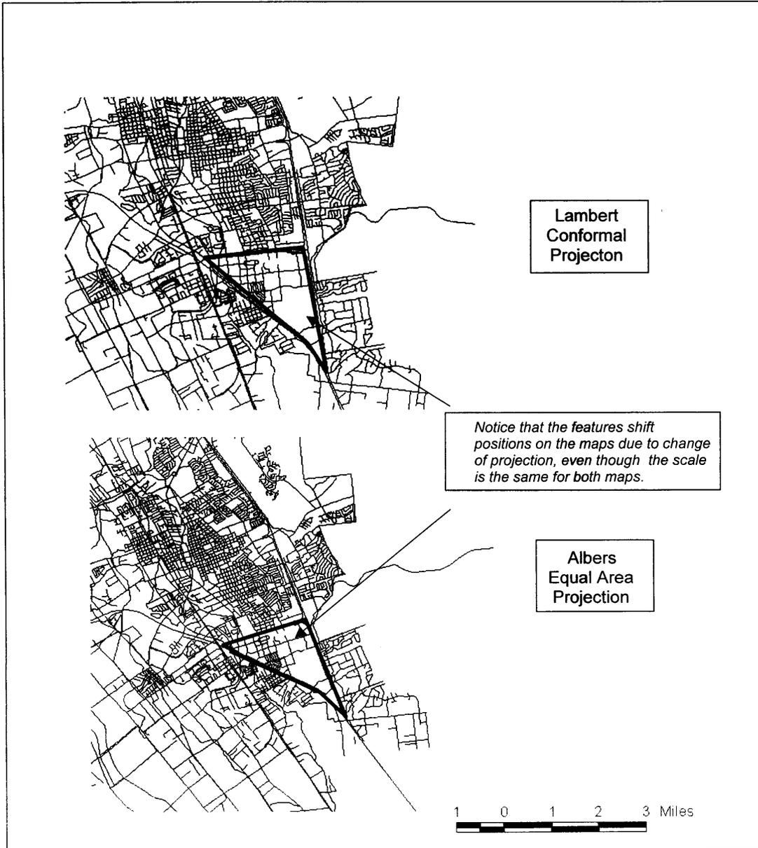
FIGURE 8 Effect of projection on the relative position of features.
