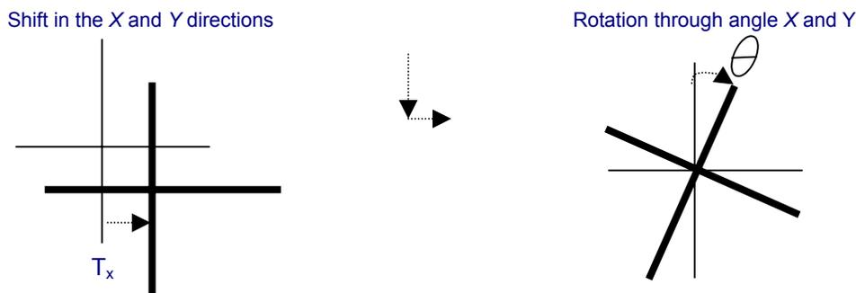
FIGURE 15 Shift and rotation as map adjustment techniques.
