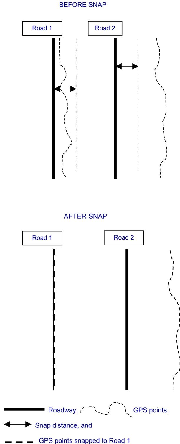
FIGURE 12 Data smoothing—Example of a snapped line.
