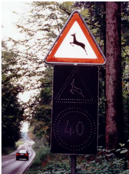
FIGURE 22 Swiss warning sign that illuminates when animals are present near the highway.
