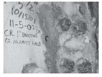
FIGURE A8 Magnetic particle testing-Indication.
