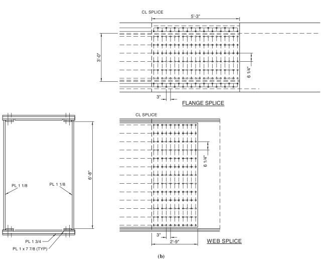
FIGURE 10 Examples of internally redundant members: (*a*) riveted built-up girder and (*b*) bolted built-up tie girder proposed for Blennerhassett Arch Bridge. (*Courtesy:* Michael Baker Jr., Inc.)
