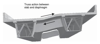
FIGURE 12 Schematic of twin composite tub girder superstructure showing internal redundancy provided by bracing system and possible alternative load path provided by slab and diaphragm. (*Courtesy:* HNTB.)
