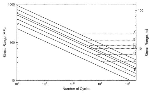
FIGURE A1 Lower-bound *S*–*N* curves for seven primary fatigue categories from AASHTO specifications. Dotted lines are the constant-amplitude fatigue limits and indicate detail category.
