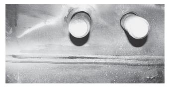
FIGURE A5 Example of indication from dye penetrant inspection.
