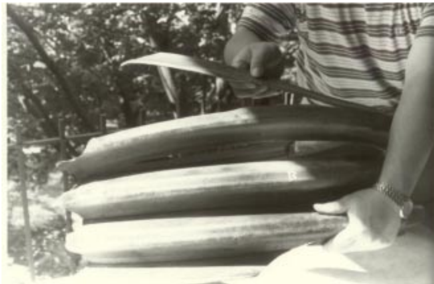
Figure 2 – A retrieved field sample containing a circumferential crack
