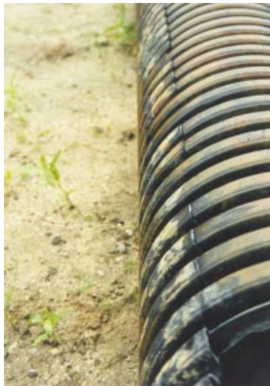
Figure 2 – A longitudinal crack along mold line in Sample J2
