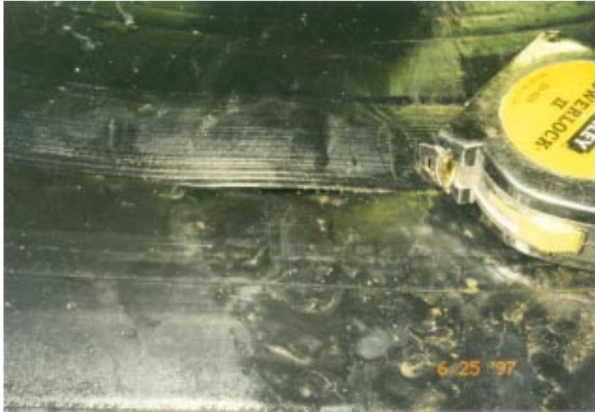
Figure 1 – Small circumferential crack in Sample H1
