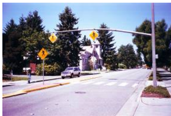
(b) Overhead Sign and Pedestrian Median Refuge Island at a Marked Crosswalk
