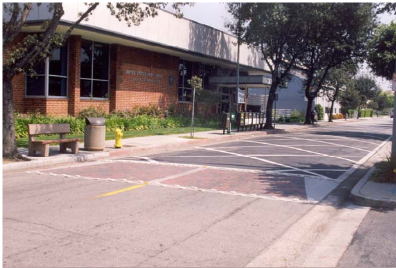
Figure D-9. Crosshatched Crosswalk Markings in Arcadia, California. (Source: Ed Cline, Arcadia, California, U.S.A.)
