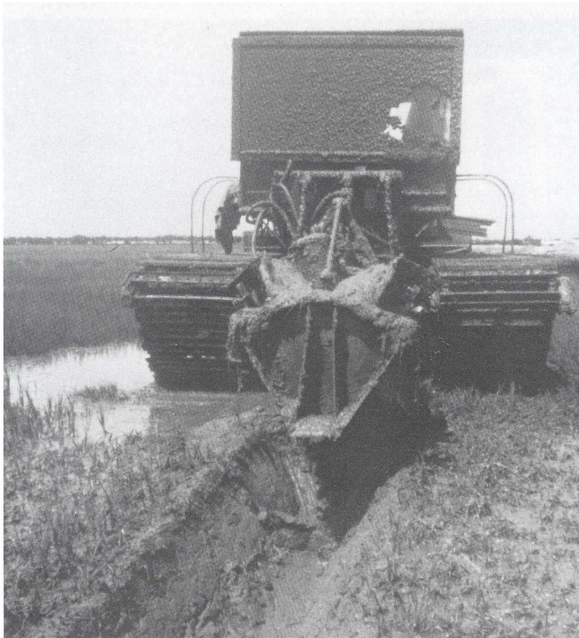
Amphibious rotary ditcher used in mosquito control can simultaneously traverse and ditch salt marshes.
