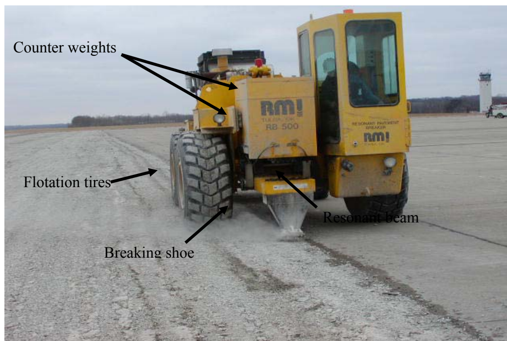
FIGURE 1 Resonant concrete pavement breaker.
