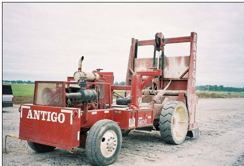
FIGURE 6 Guillotine style breaker.
