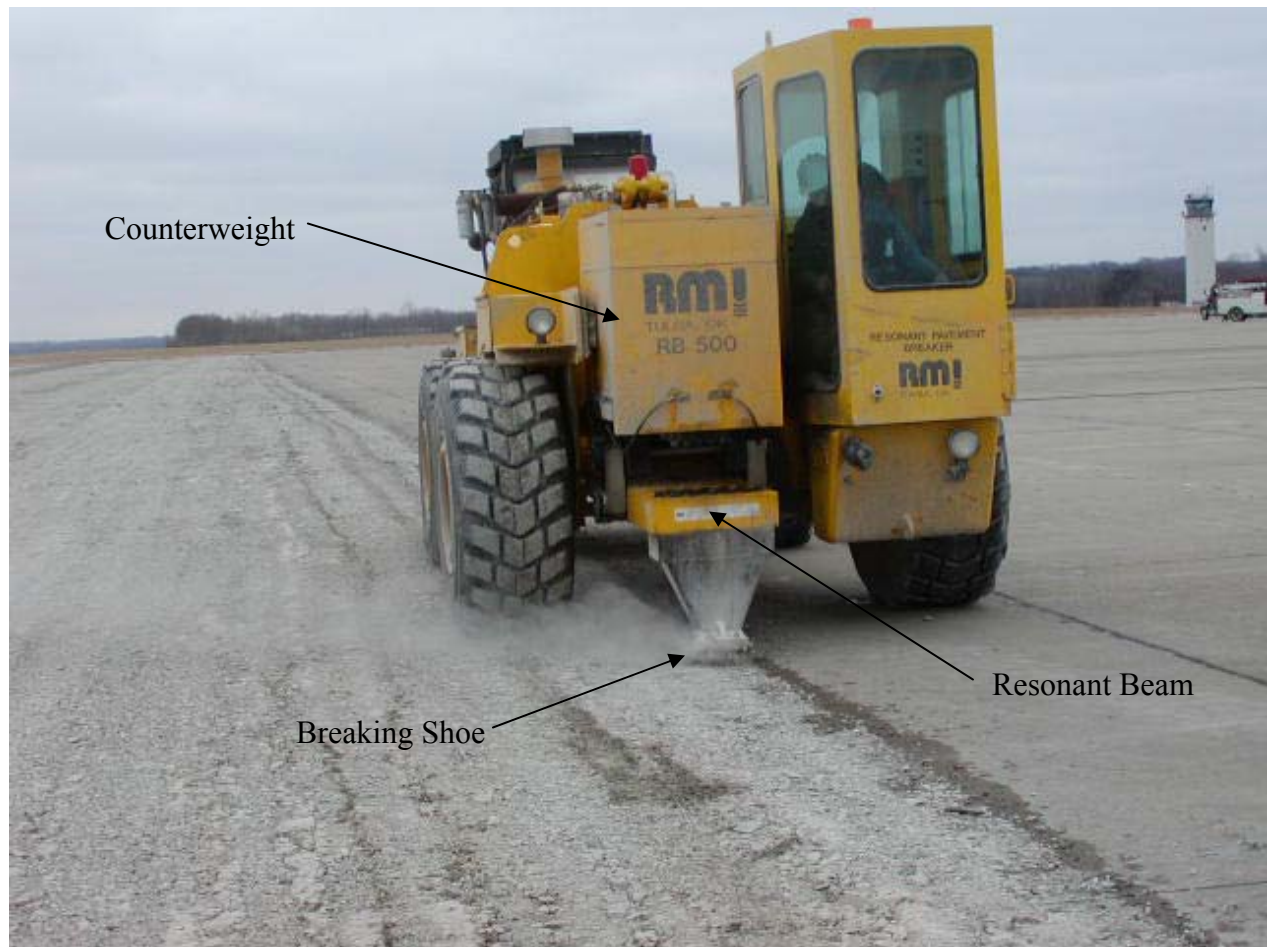
FIGURE 1 Resonant pavement breaker (courtesy RMI, Inc.)
