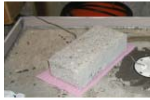
Brick with insulation on bottom surface to secure thermistor to pavement sensor
