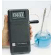
Thermometer and thermistor to check air/pavement temperature
