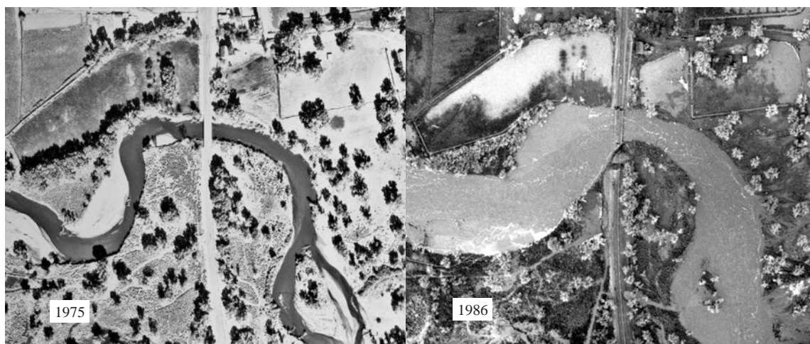
Figure 1.2. The US-95A bridge over the Carson River near Weeks, Nevada, in 1975 and 1986. Significant meander migration during the 1986 flood caused severe erosion of the south embankment and flanking of both bridge abutments, which ultimately resulted in failure of the bridge.
