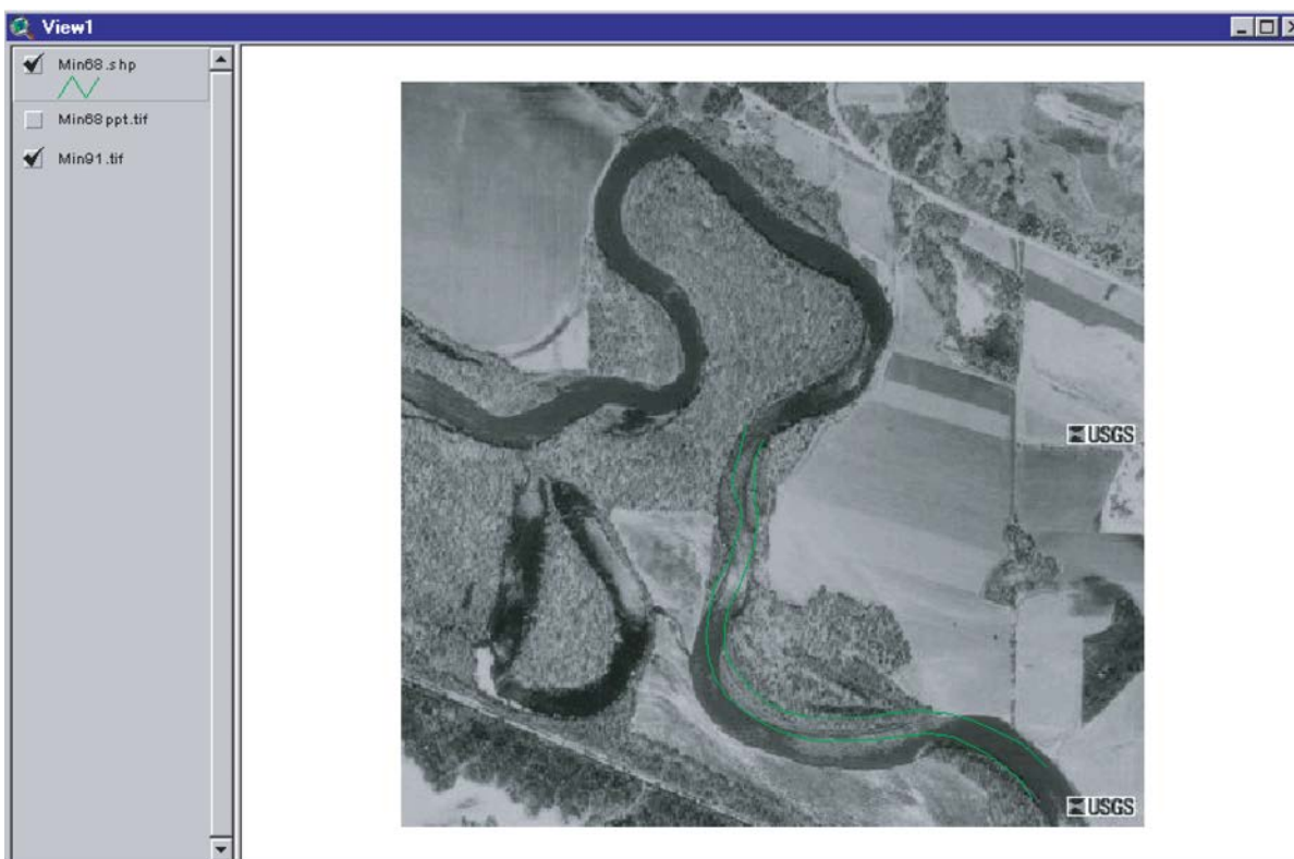
Figure D.5. 1968 banklines after being turned into a Shapefile and superimposed on the 1991 reference photo.
