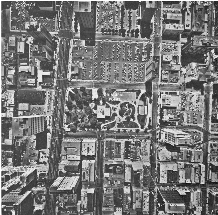
Figure 4.1. Vertical aerial photograph illustrating relief displacements.
