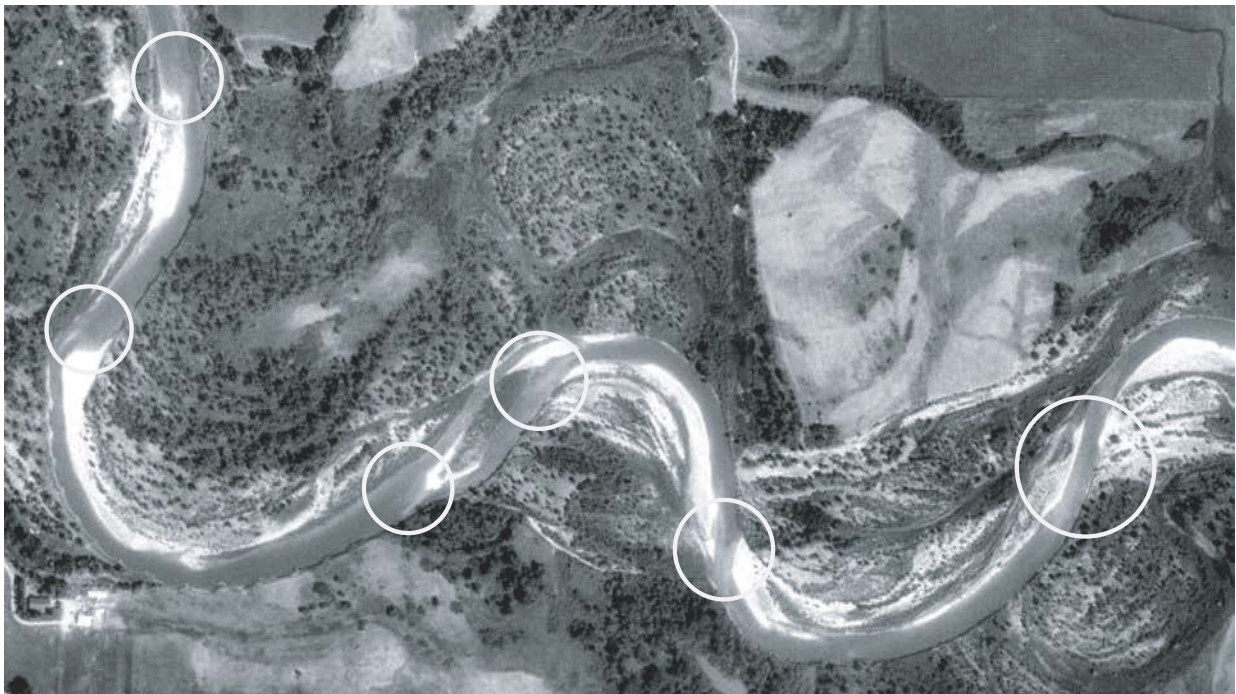
Figure B.12. Aerial photo of the gravel-bed Sun River in Montana showing the locations of several riffles identified by circles.
