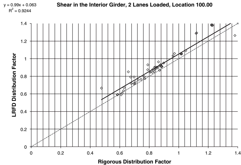
Figure 95. Spread box beam, shear, interior girder, two lanes loaded (example of a regression plot).
