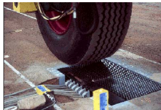
FIGURE 2 The VRSPTA on the pavement under the HVS with a 315/80 R22.5 tire (De Beer et al. 1997).
