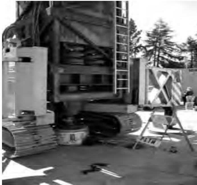
Figure 120. Illustration of the Pseudo Static Pile Load Tester (Schellinghort, 1996, Coe.Berkeley Website)
