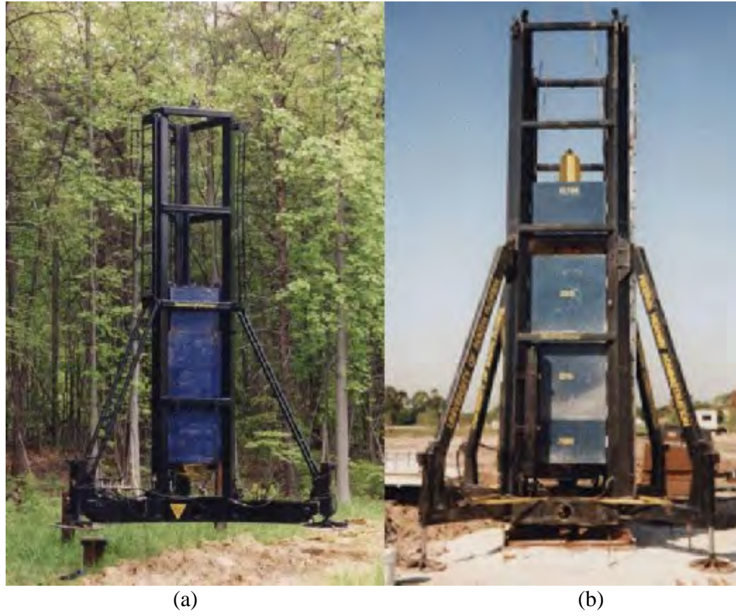
Figure 30. (a) 0.6 MN device, and (b) 4 MN device utilizing mechanical and hydraulic catch mechanisms respectively
