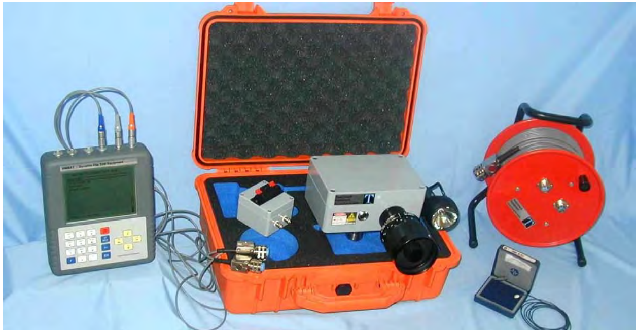
Figure 94. The Components of the SIMBAT System (Testconsult Website)
