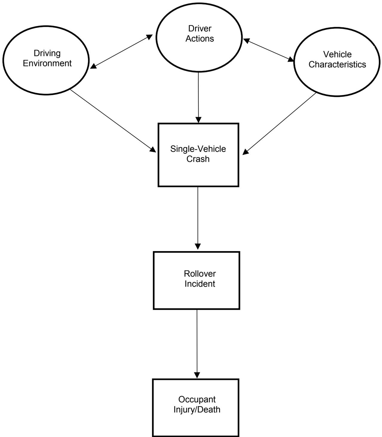
FIGURE 1. Interactions that result in single-vehicle rollover crashes.
