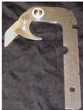
Figure 1 Standard AAR wheel gauge
